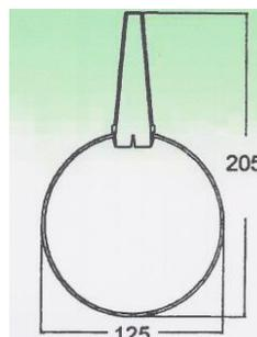
Pipe with, on the upper side, little pipes of +/-80mm high, every 50mm. Straw and big parts of dirt can't go through these little pipes, so the pipe can't block up. This drainage system is suitable for spaces with straw.
