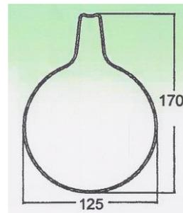
Pipe with, on the upper side, openings of  $\varnothing 10\text{mm}$  every 50mm. Straw and big parts of dirt can't go through these openings, so the pipe can't block up. This drainage system is very suitable for spaces with straw.
