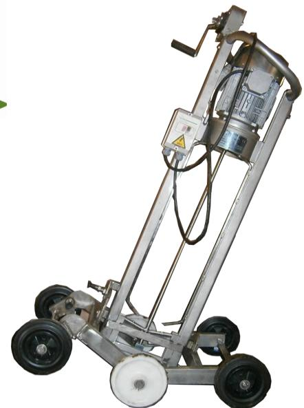
Adjustable height with brake to mix at different heights, which make work more practical and safer.
